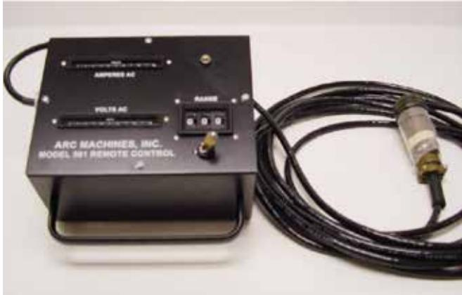
The Model 501 remote pendant is designed to allow the operator to control the hot wire output of the Model 501 hot wire power supply. The operator can set the desired output voltage via the thumbwheel potentiometer on the pendant, from 0.0 to 20.0 volts. When the operator flips the toggle switch, the output goes active.
